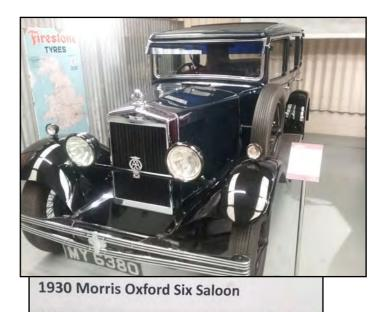
1927 saw a marked change in the styling of Morris cars, the familiar 'bullnose' radiator was replaced by a more conventional, flat type. Fitted with a six cylinder engine, this revised Morris Oxford went into quantity production the following year.
