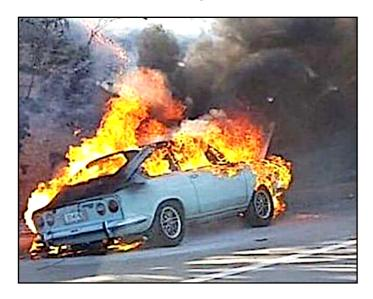
The car is a Fiat 850 Sport Coupe, rear-engined (as was the trend in Europe at the time) with the fuel tank sandwiched between the engine and the rear seat.
