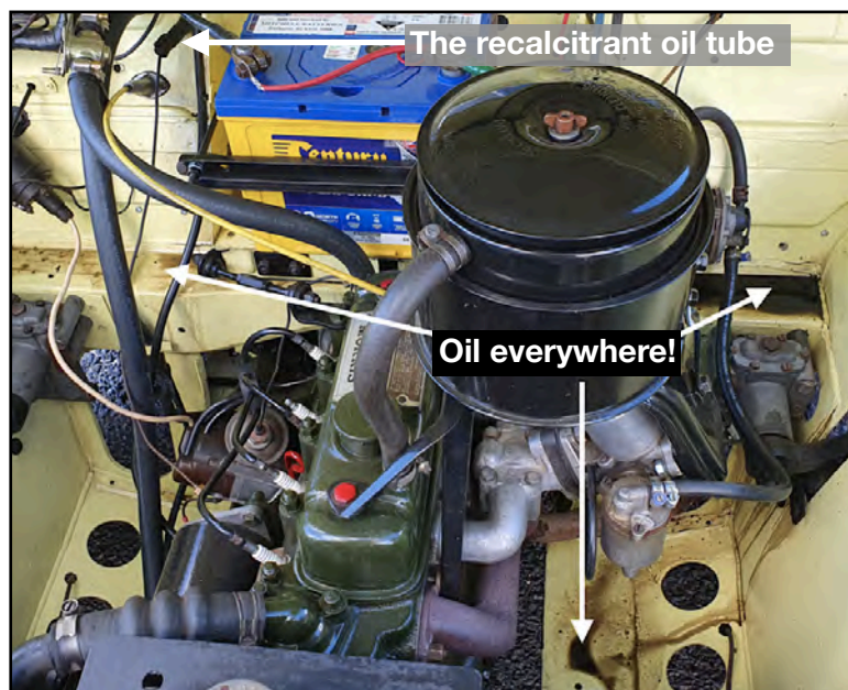
Denis Woodford's oily engine bay was nothing compared to the oil in his driver's footwell
