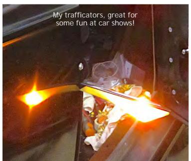
So, in October 2022, in went my trafficators which Les had reco'd with new arms ages before. And remember, he had hidden a switch under the dash to switch between blinkers and trafficators; blinkers on the road, and trafficators for a bit of fun at displays.
