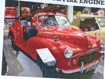
The photo above is of the fire engine built in 1953 by the Engineering Division of Morris Motors, using the prototype chassis for the new quarter-ton Morris Minor van. It was originally fitted with the side valve engine, but was later converted to the more powerful overhead valve "A" series engine.
